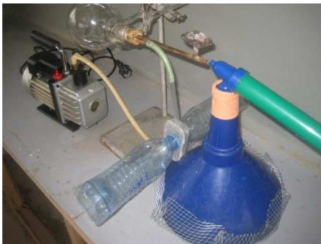
*Figure A1. Nose-only Smoke Inhalation Apparatus.*
